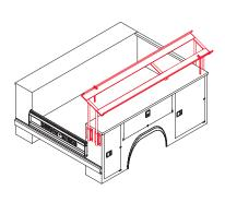
LRF - Ladder Rack (Side Mounted, Flat Type)
