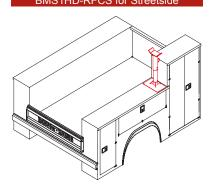
Crane Boom Support BMS2 for 14 1/2 " Compartment Depth BMS3 for 20" Compartment Depth
